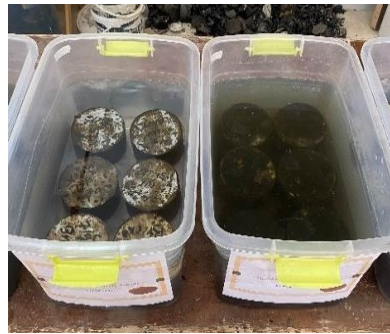
Fig.4: Immersed sample in fresh and sewage water
